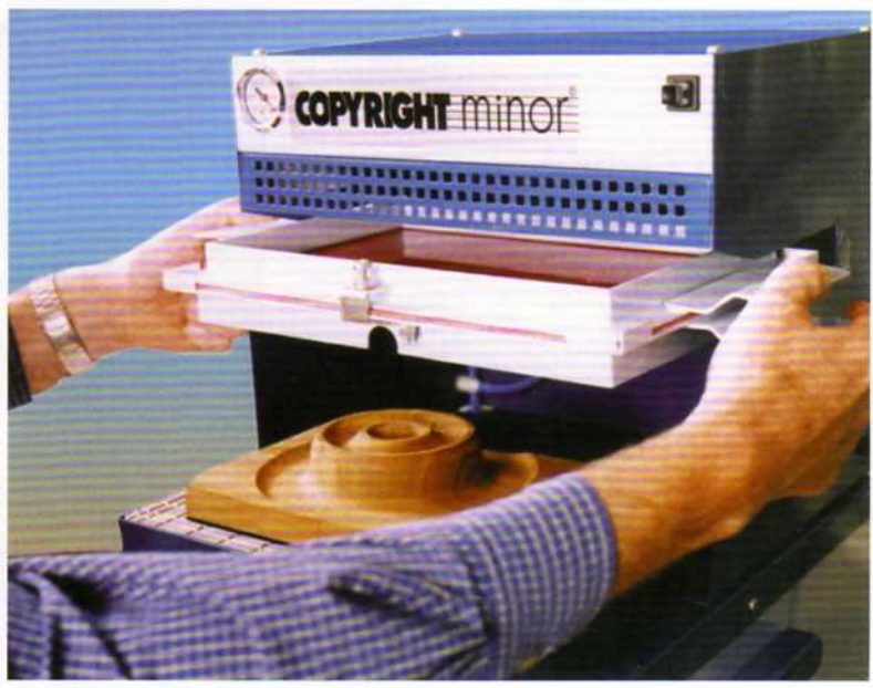
1) Upper and 2) Lower forming frames for positive location of plastic
